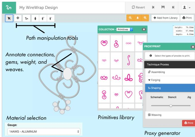
**Figure 4.** The ProxyPrint digital design tool for wire forms. Users can drag common forms onto a canvas, manipulate paths, specify materials, and add ornamentation and connections. The tool produces a heightmap used to generate a 2.5D printable proxy.
